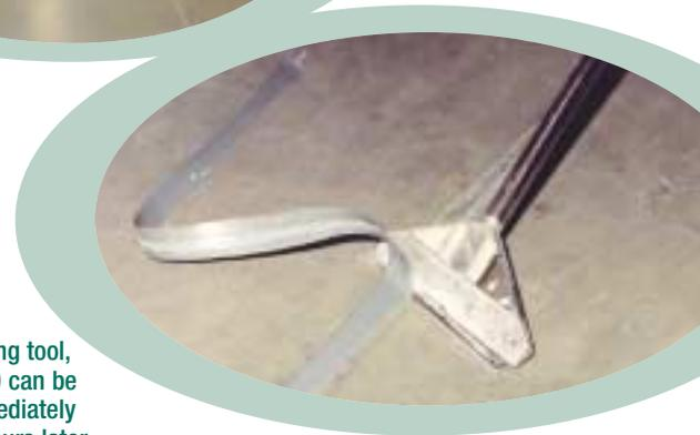
Using a shaving tool, QWIKjoint 200 can be trimmed immediately or up to 24 hours later.
