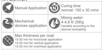
The substrate must be perfectly clean, compact, free from dust, grease, paint, etc. Carefully remove the deteriorated and flaky concrete using a hammer until the substrate is compact.
