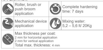
The substrates must be clean and mechanically consistent, any holes or irregularities in the substrate must be previously repaired with suitable Kimia products. In case of waterproofing of already tiled surfaces, remove the first row of wall tiles for a height of about 20 cm, perform an acid washing of the surface with **Soluzione P**.
