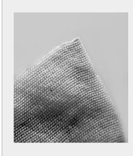
Pre-primed, alkali-resistant polypropylene reinforcing fabric for waterproofing and protective cycles
